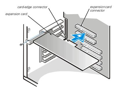
Figure 8-4. Installing an Expansion Card
